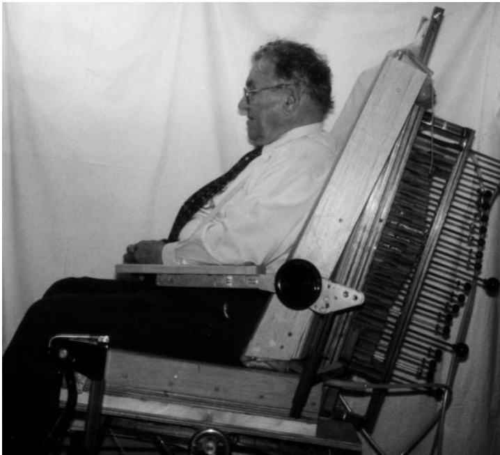
Figure 2-19: The developed fitting chair with central support of the spinal column by means of rectangular elements. Notice how the curvature of the spinal column can be seen at the back of the chair.
