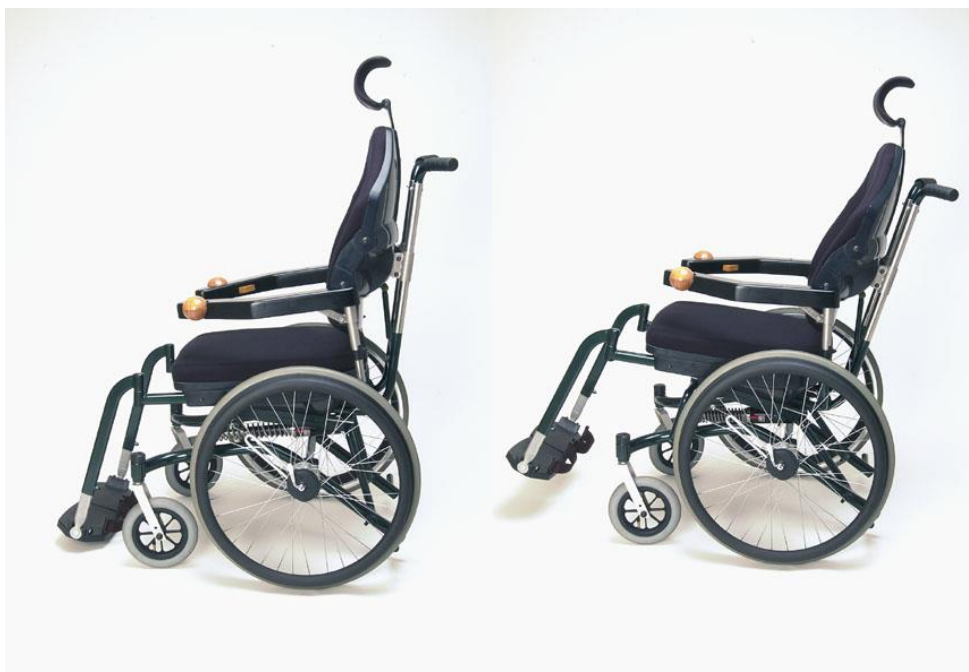
Figure 4-27: Non-folding wheelchair C-Rex with electrically driven tilt adjustment and individually adjustable back support: in the transfer position and in a position for a stable sitting posture.
