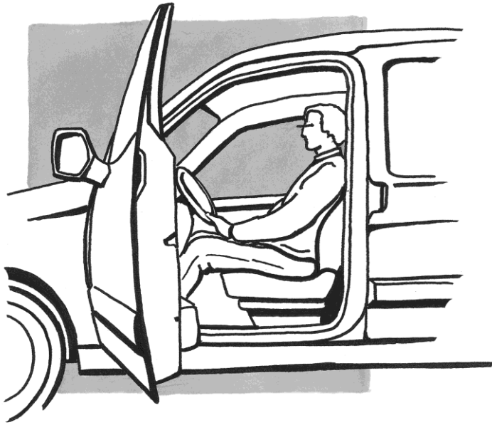
Figure 3-30: The individually preferred posture with the head in balance on the trunk as seating posture in a vehicle with a functional backrest angle: angle( \varphi+\alpha ) of ca. 123°.
