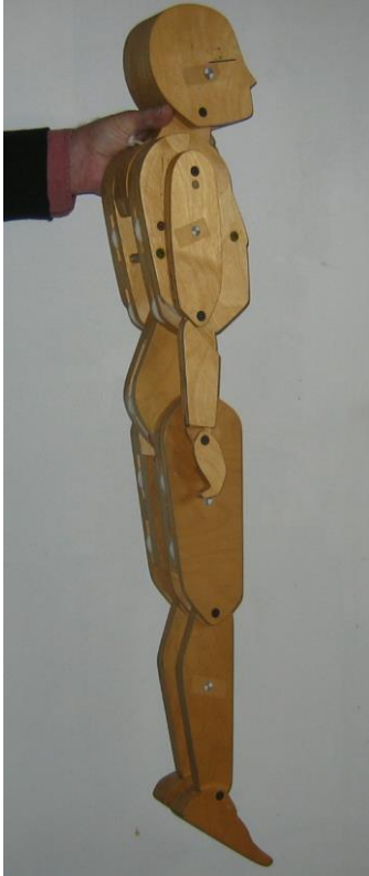
Figure 2-14: 3D loose-jointed test dummy with tiny wheels in thighs and back to enable demonstration of stability and frictionless sitting.
