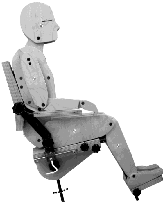
Figure 2-18: Loose-jointed test dummy in stable sitting posture without friction on the seat or backrest.
