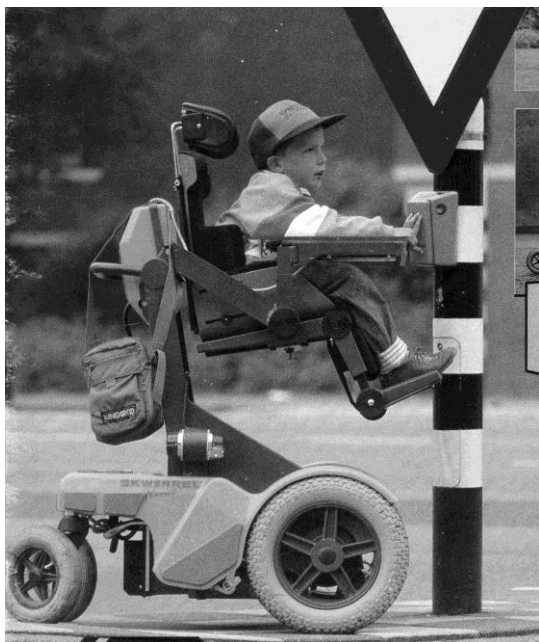
Figure 4-21: The Squirrel: a children's electrically driven wheelchair with vertical and tilt adjustment.
