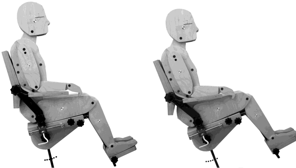
Figure 4-5: From the basic posture to the individually preferred posture: angle( \varphi+\alpha ) from 116^\circ to 123^\circ .
