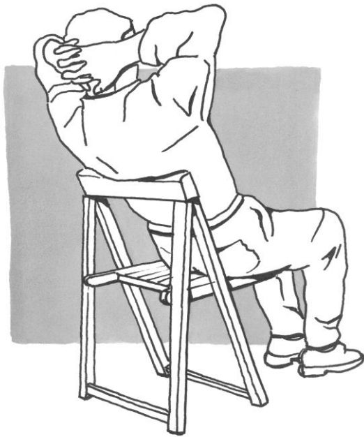
Figure 4-9: Supporting the head in a posture with functional backrest angle, angle( \phi+\alpha ) > 123° to compensate for extra muscle exertion in the neck and shoulders.
