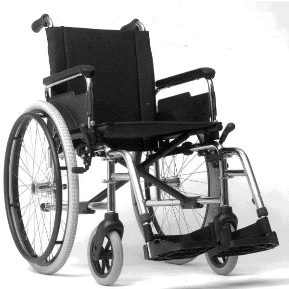
Figure 4-28: Traditional folding wheelchair: optimised for transfer and suitable for very short periods of use. The seating angle, angle \varphi is approximately 0^\circ , the backrest inclination, angle (\varphi+\alpha) is approximately 105^\circ .
